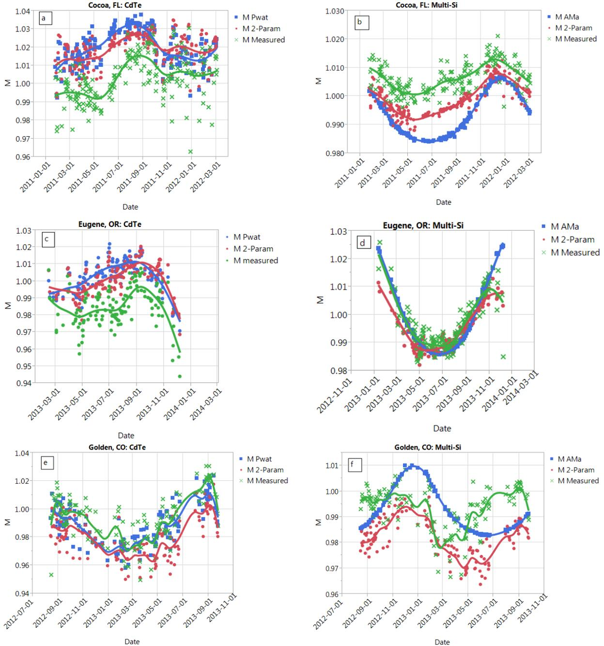
Fig. 3. Time series of measured and modeled  $M$  for: a) CdTe module at Cocoa, FL; b) multi-Si module at Cocoa, FL; c) CdTe module at Eugene, OR; d) multi-Si module at Eugene, OR; e) CdTe module at Golden, CO; and f) multi-Si module at Golden, CO. For the CdTe modules,  $M$  was estimated using the (1) and the  $P_{wat}$ -only spectral corrections. For the c-Si modules,  $M$  was estimated using the (1) and the  $AM_a$ -only spectral corrections.
