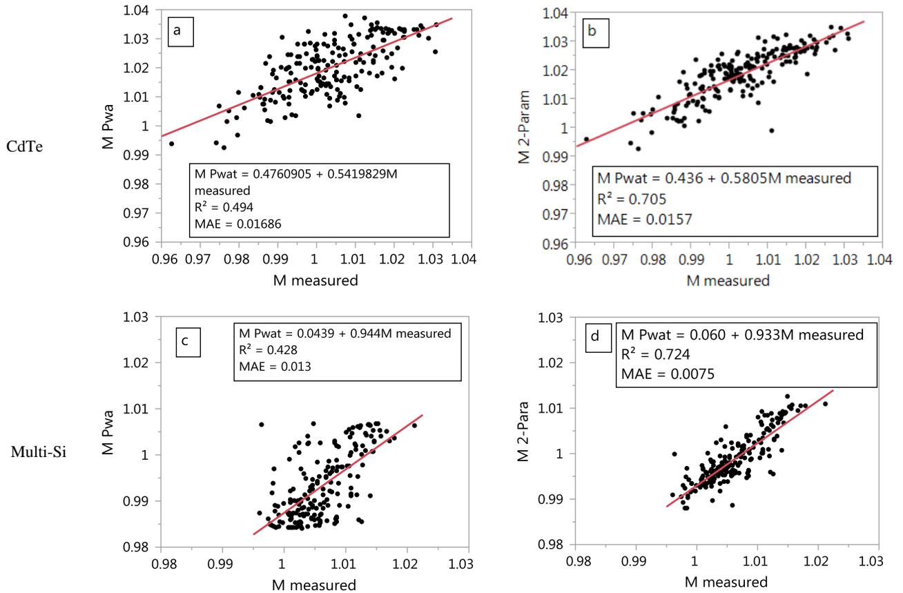
Fig. 2. a) CdTe spectral correlation proposed by [1] versus measured  $M$  for the CdTe module. b)  $M$  estimated using (1) versus measured  $M$  for the CdTe module. c) “Sandia” spectral correction [7]-[8], versus measured  $M$  the multi-Si module. d)  $M$  estimated using (1) versus measured  $M$  for the multi-Si module. All  $M$  data is of daily resolution and GHI weighted.
