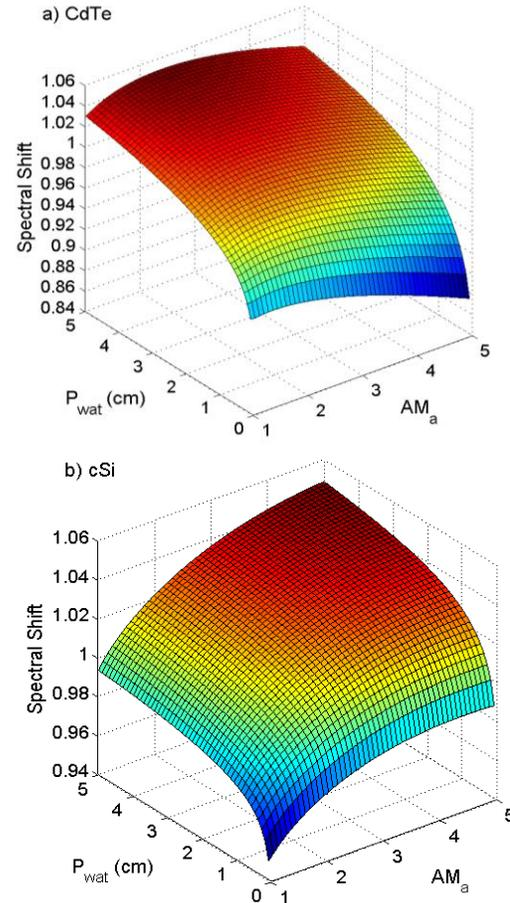
Fig. 1. Sensitivity analysis of  $M$  as a function of  $P_{wat}$  and  $AM_a$  for a) CdTe and b) multi-Si.
